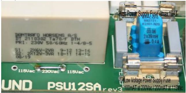
The Low Voltage Supply on PSU12SA has two options of Mains Voltage selection: 230Vac and 115Vac.
