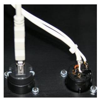
The **Function Switch** for AUTO-OFF-ON on PSU4SA/PSA12SA wire will be sufficiently wired with 0,2mm<sup>2</sup>. This is a low current wire and it's no problem with 1m wires, if it is desired. Example: Mounting on front panel.
