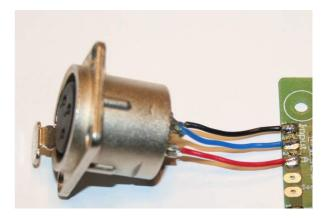
The **CH** pad on DCN23/24 is actually the ground lifted connection of the system which should be wired to chassis metal very near (RCA) or on the input connector (the Neutrik XLR connector has a soldering tag for this purpose).
